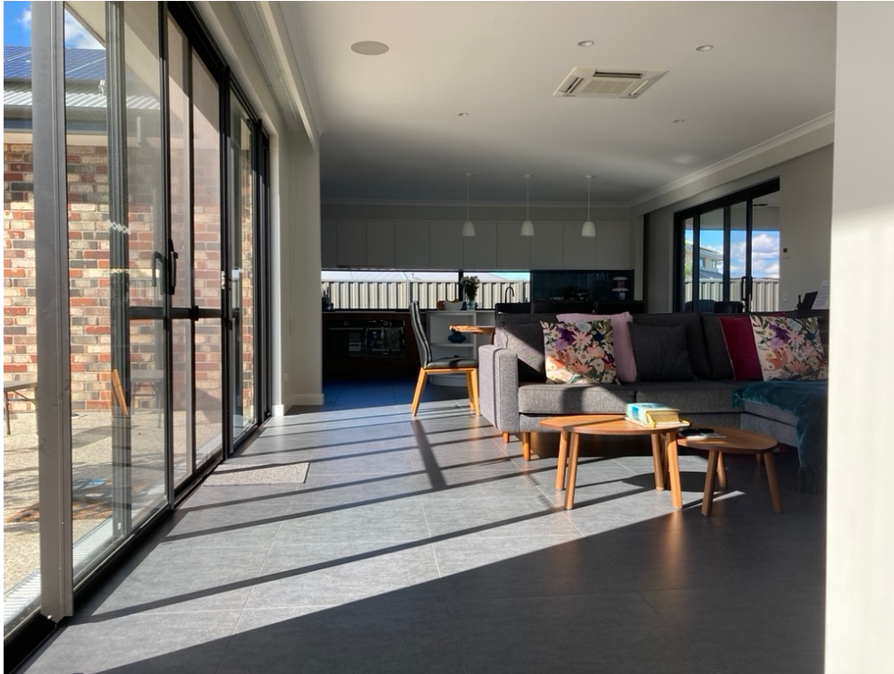
Image 3: North-facing windows allow Winter sun to penetrate deep into the floorplan, providing residents with free heating and increased comfort on a Winter's day. Excluding Summer sun from the North is simple with a correctly-sized eave or horizontal shade. Image courtesy of author.
