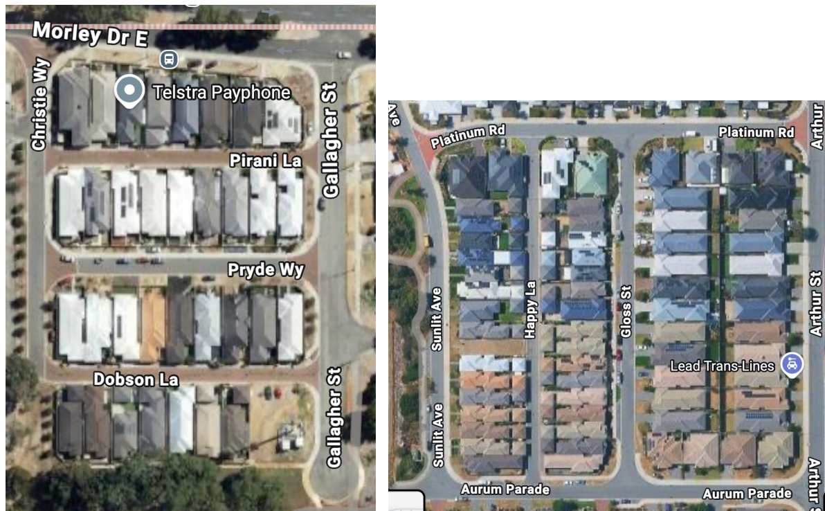
Image 1 and 2: Examples of developer-volume builder housing from Perth's eastern suburbs, showing lack of care regarding site orientation, established tree canopy on development fringes only, and very little vegetation within the development. Often the greenery shown in satellite images is artificial grass. Perth had 16% tree canopy coverage in 2020; this percentage has continued to decline 6 . The first image is in Eden Hill, the second in Dayton, images from Google Maps.
